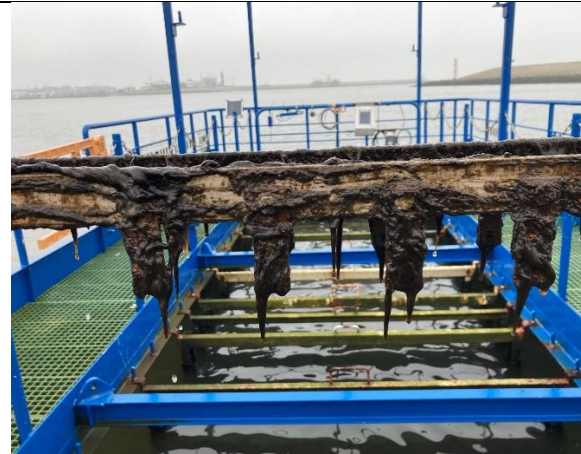
Figure 20. Rack mounted with metals after 3 months of immersion in the seawater at the raft (detailed).
