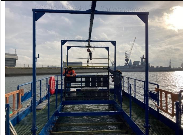
Figure 6. Metal framework on the raft to mount samples.
