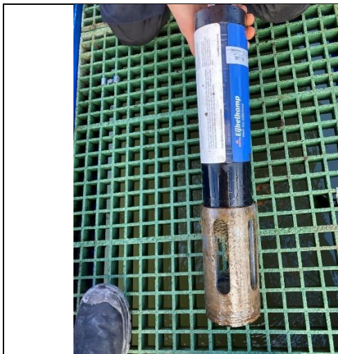
Figures 21 and 22. Environmental sensor after 2 months of exposure.
