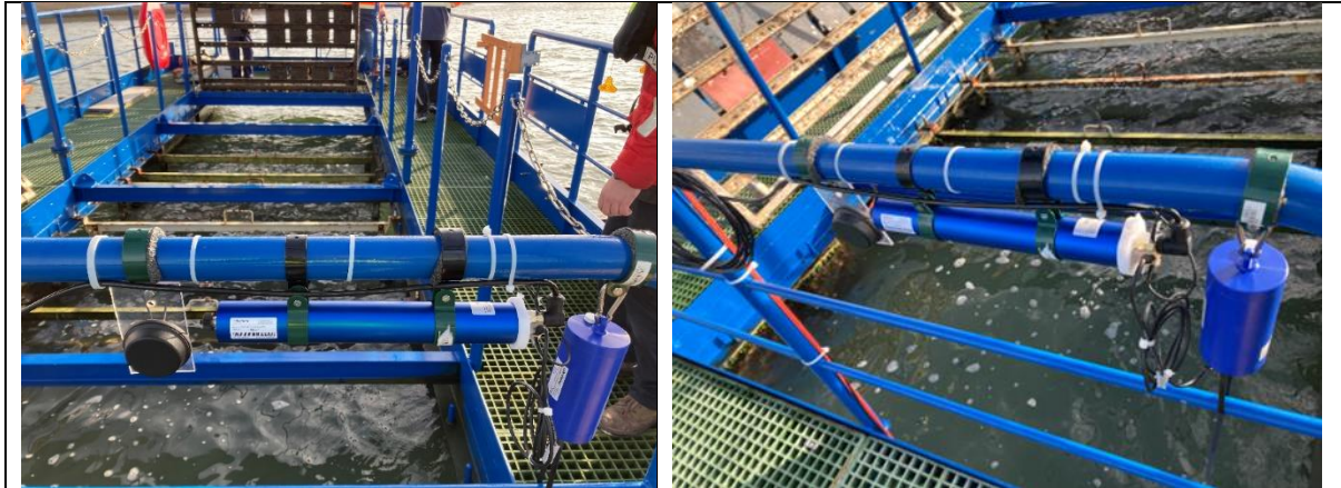
Figure 12-13. Mounting the battery pack and wifi module of the environmental sensor on the raft infrastructure.
