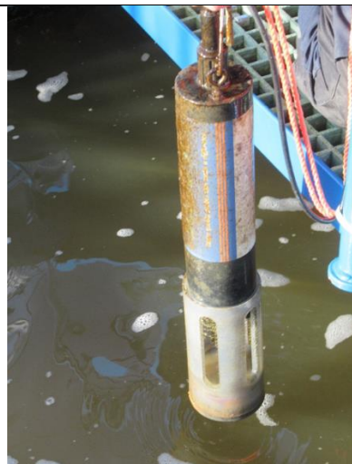
Figures 21 and 22. Environmental sensor after 2 months of exposure.
