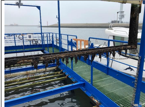
Figure 19. Rack mounted with metals after 3 months of immersion in the seawater at the raft
