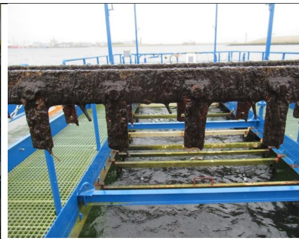
Figure 18. Rack mounted with metals after 2 months of immersion in the seawater at the raft (detailed).
