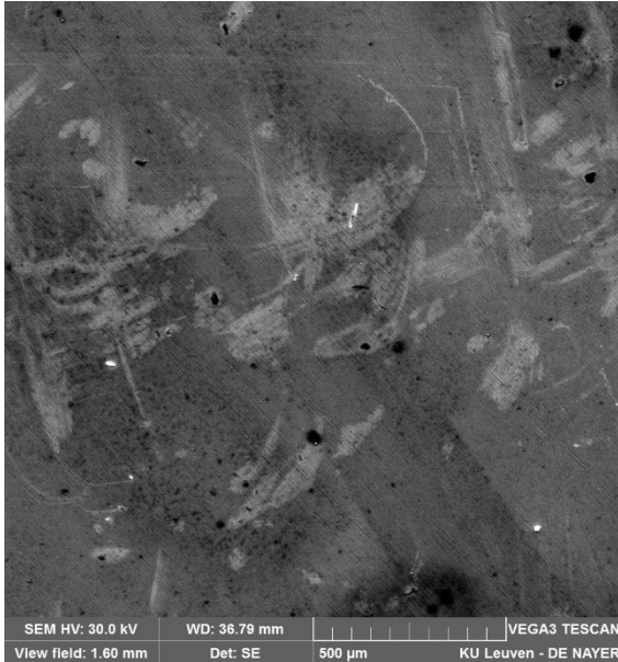
Figure: No pitting corrosion found after polarization in the PB Leiner wastewater for DX2205.
