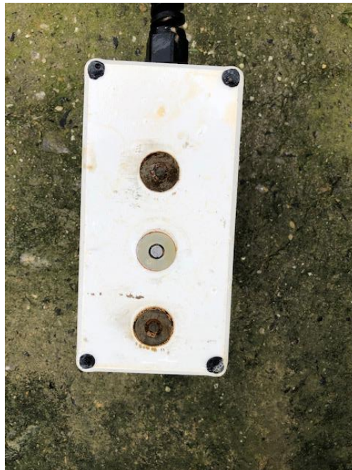
Figure: The C-Cube LPR probe after being in the wastewater of PB liner for 2 months without any cleaning.
