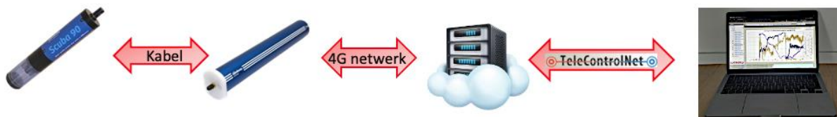
Figure 7. Overview of how data flows from sensor to web portal
