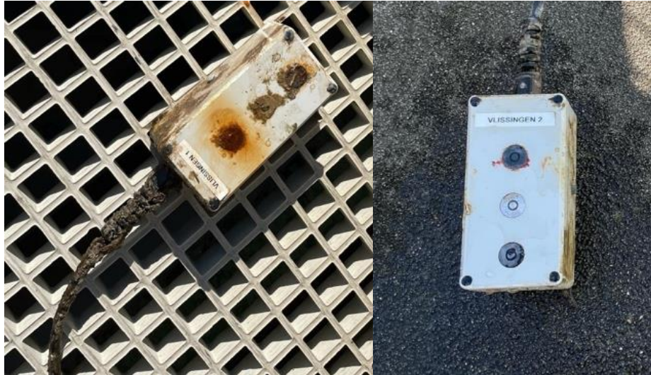
Figure 20. CCube probes at VL1 (left) and VL2 (right) before re-installation
