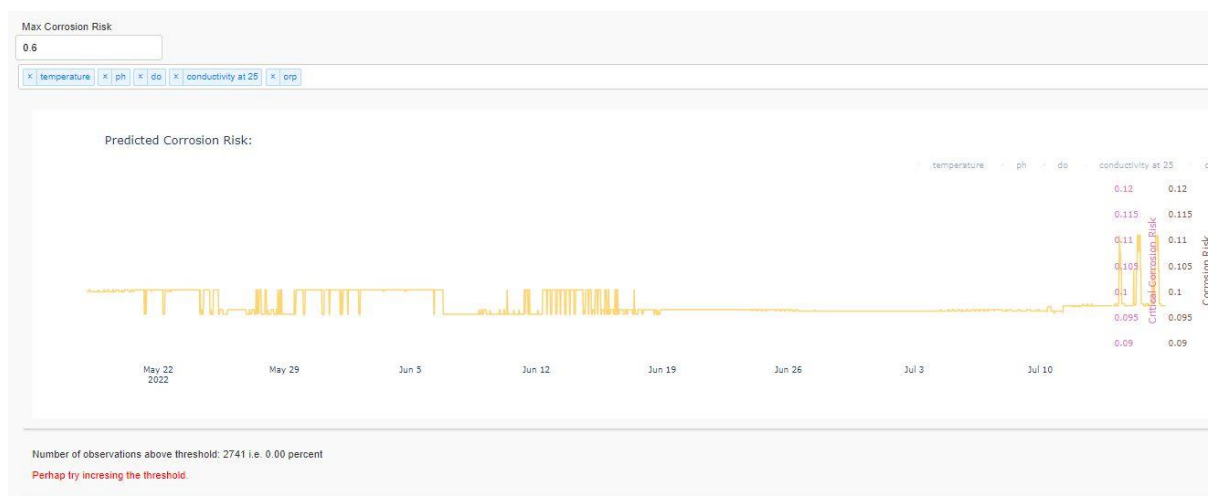
Figure 39: BLUE2, Measurement Campaign 1, Corrosion Risk as calculated using the SOCORRO Application (model trained using Field data). Threshold set at 0.6.
