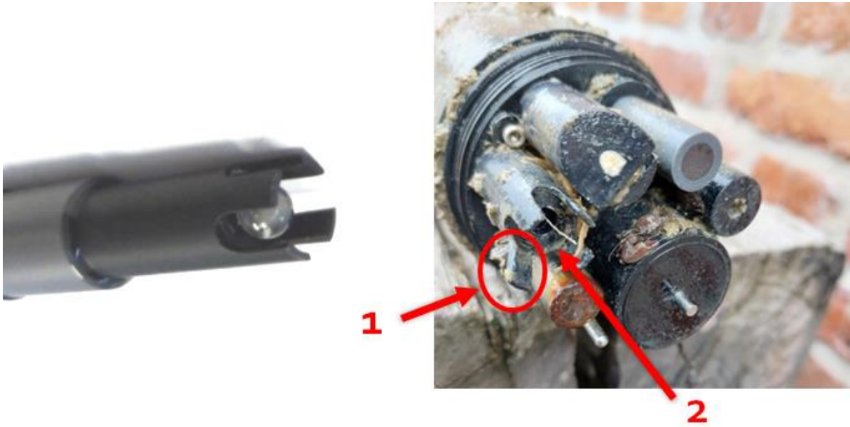
Figure 10: Left: pH probe in new condition with clearly visible glass sphere as sensor element. Right: Multisensory probe after retrieval on 10/10/2022. [1] Bent plastic protection leg. [2] Glass sphere missing.
