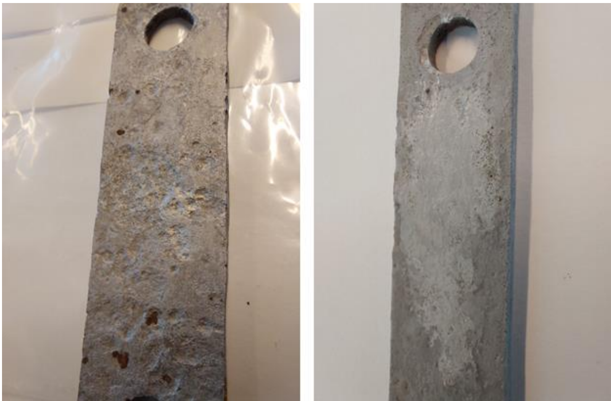
Figure 18: Left: coupons exposed on the outside of the monopile for 147 days. Right: coupons exposed on the inside of the monopile for 254 days.
