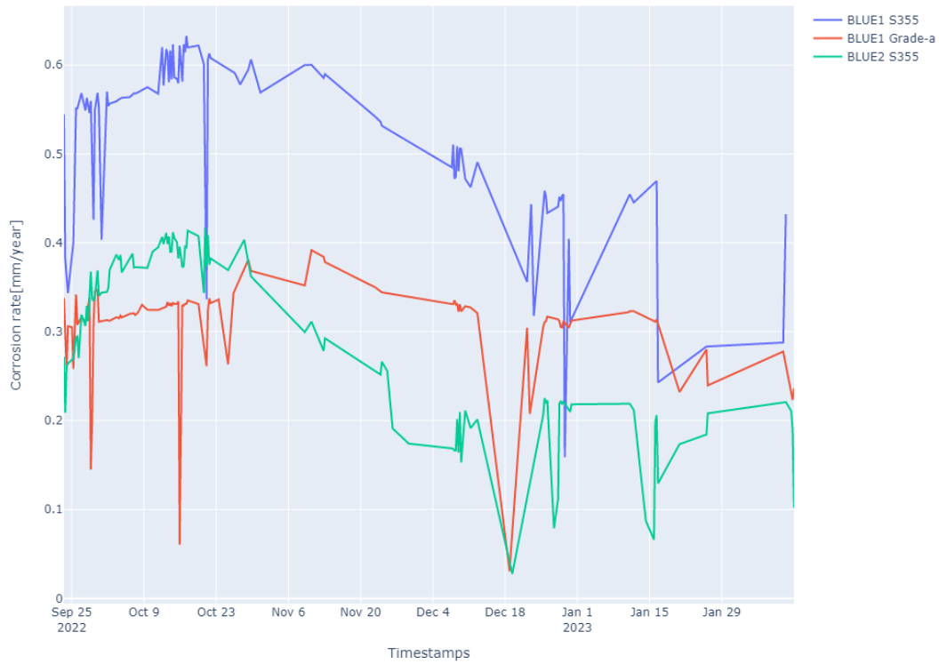
Figure 15: C-Cube corrosion rates. Internal (BLUE1) vs. external (BLUE2) corrosion.
