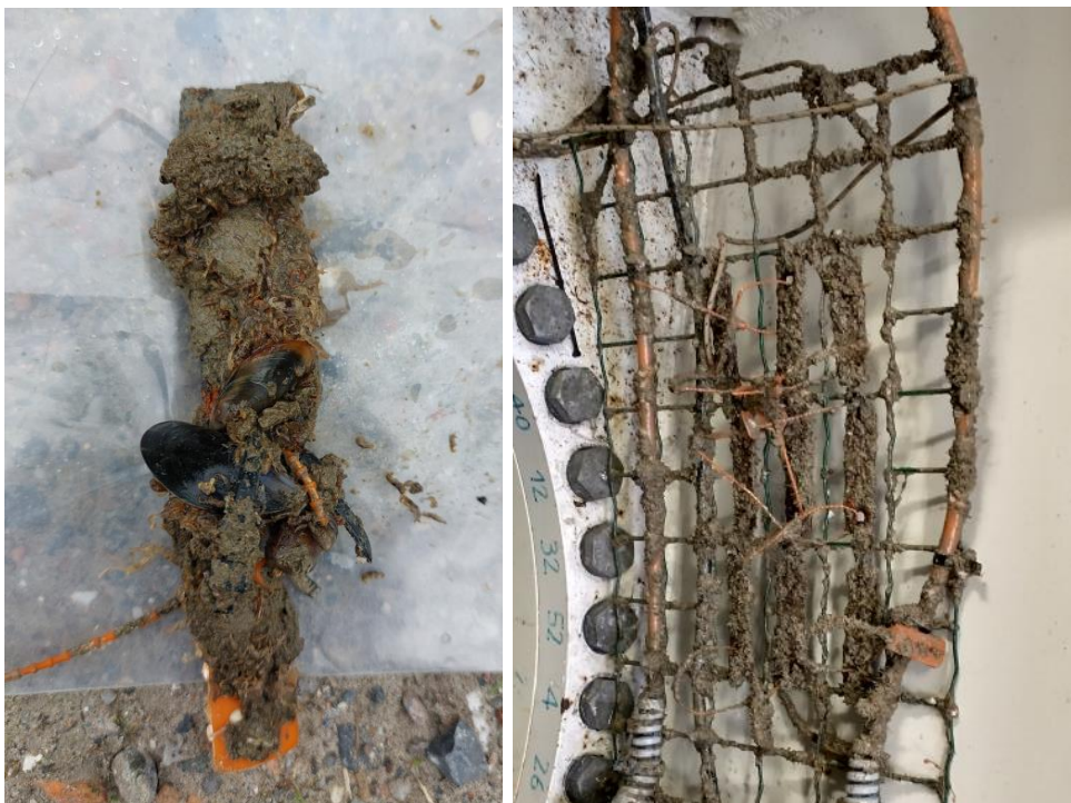
Figure 20: Illustration of fouling on corrosion coupons. Left: external; Right: Internal.
