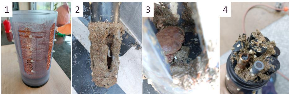
Figure 9: [1] Picture of a new protection cap with copper mesh present (fortified version for measurement campaign 2). [2] Presence of fouling on sensor during inspection on 10/10/2022 (BLUE2), with copper mesh clearly missing. [3] Presence of a large crab within the sensor protection cap. [4] Significant fouling on the sensors themselves.
