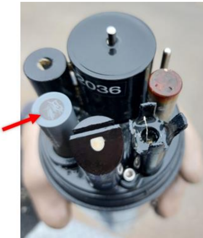
Figure 11: Scratch marks on Chloride ISE sensor.
