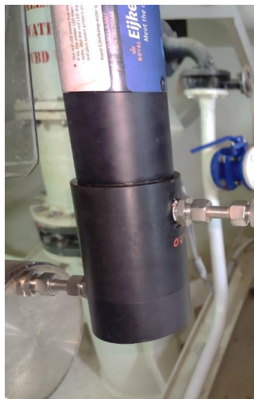
Figure 4: Specially designed flow cell (end cap).
