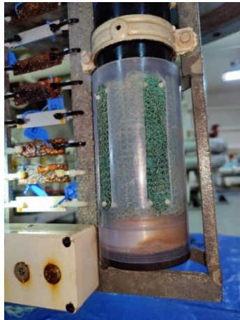
Figure 3: End cap with openings on the side.
