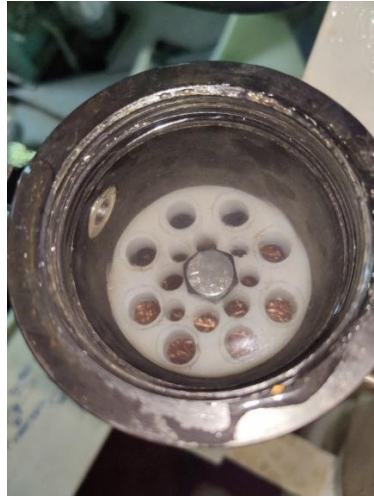
Figure 5: Copper mesh in the flow cell.
