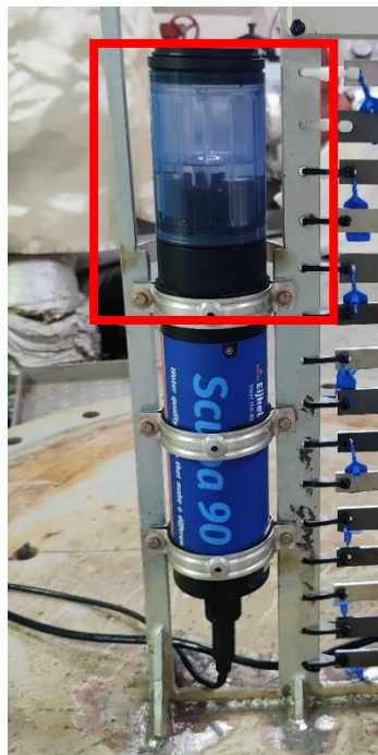
Figure 2: Storage cap on the Scuba probe.
