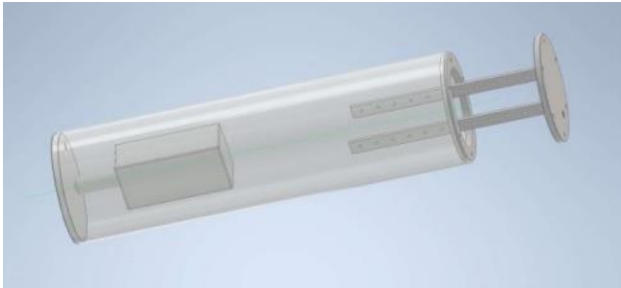
Figure 29: Flow cell for the C-Cube sensor and corrosion coupons.
