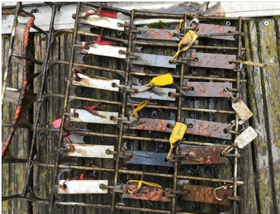
Figure 20. Coupons after 1 month exposure in Zelzate North (February 2023). Yellow labeled plates are S355 alloy and white labeled plates are the S235 alloy. Red labels indicate 316L.
